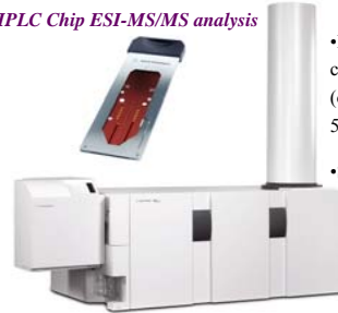
Figure 2. The Agilent 1200 HPLC-Chip MS/MS system equipped with an 6510 QTOF was used for the nano reversed-phase HPLC-ESI-MS/MS analysis.
